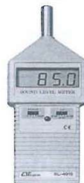
Figure (4): Pre-Calibrated Sound Level Meter At 114 dB(A)
